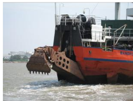
Figure 1 Self-propelled hopper dredge ship during operation
