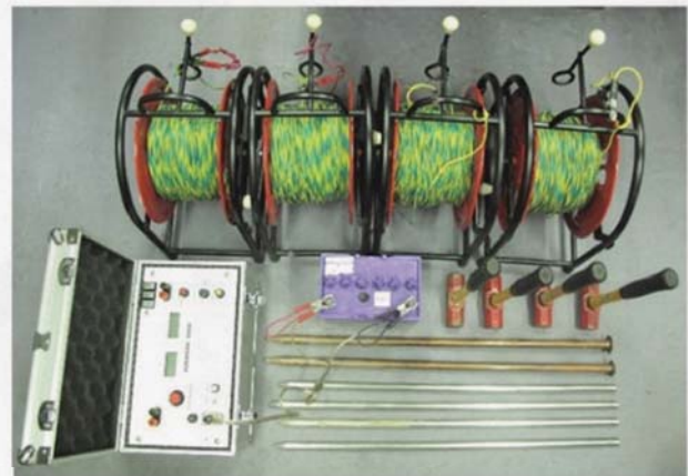
Resistivity meter and equipments
