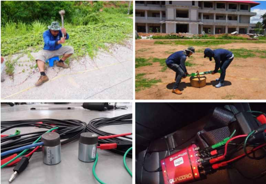
Figure 5. Equipment used for SASW measurement (a) Sledgehammer (b) drop weight (c) two geophone receivers (d) spectrum analyzer
