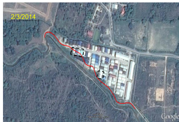
Figure 16 : Lateral spreading observed at new filled soil area
