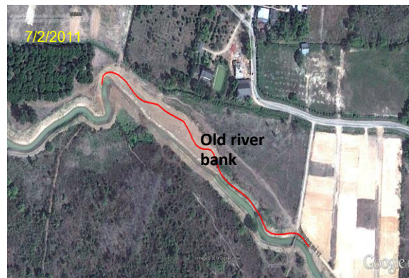
Figure 15 : Lateral spreading observed near the river or stream channel
