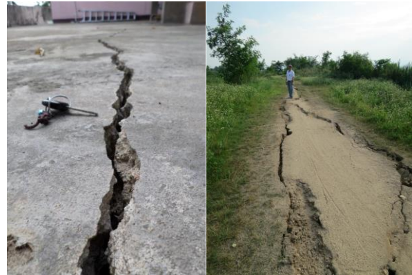
Figure 15 : Lateral spreading observed near the river or stream channel
