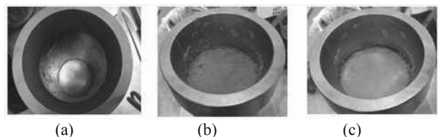
Figure 5. (a) Strips inside the interior wall of the mold; (b) 2300g of wet soil were placed in the mold, and, (c) A plastic circle was placed on top of the mold for the soil not to stick to the compaction platen.
