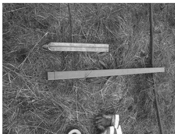
Figure 8 Inclinometer tube of PVC with square cross-section with steel point at the end.
